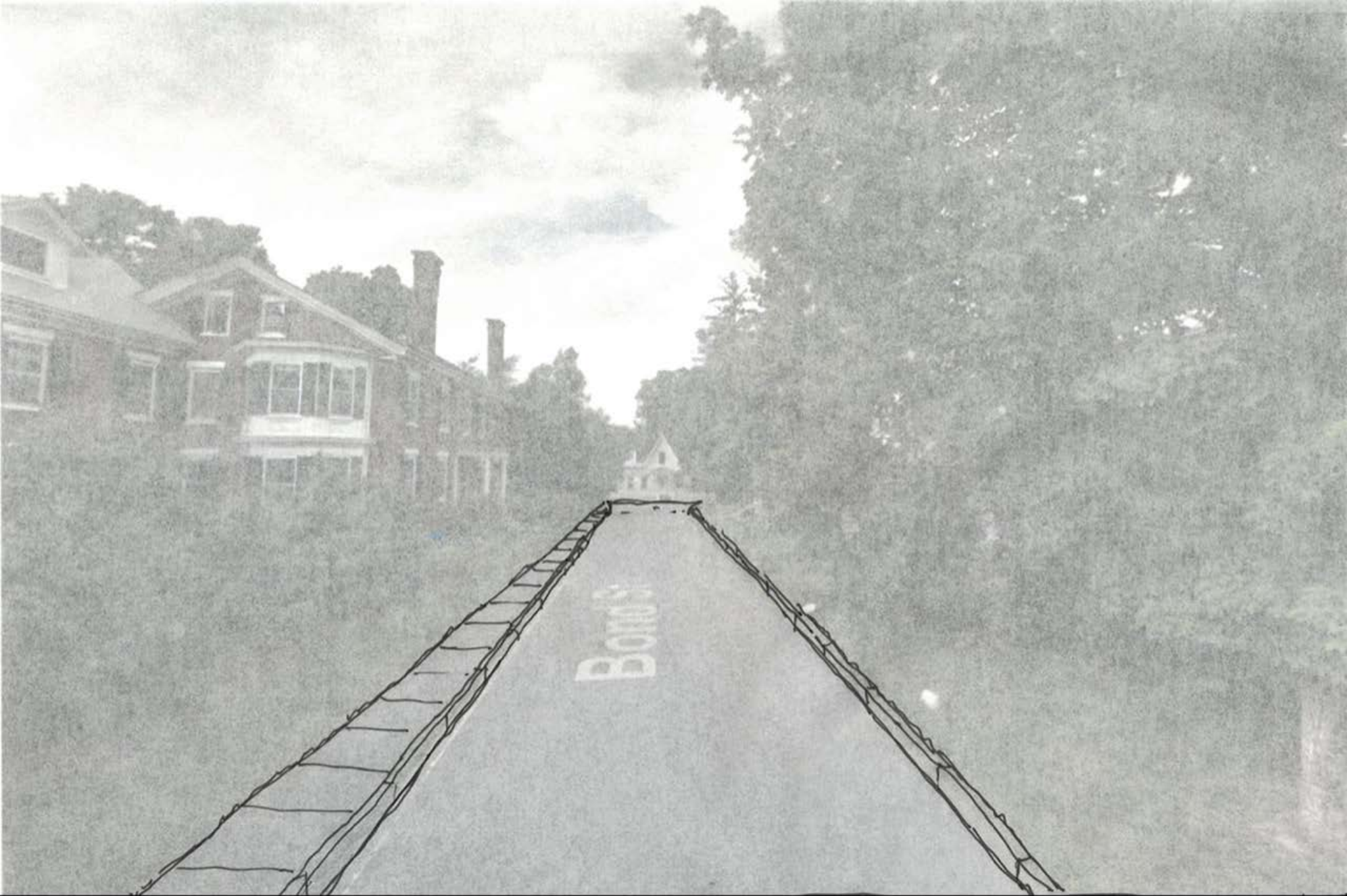
2013 view of Bond Street looking north, with sketch of proposed curbing and sidewalk.
